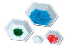
Hexagonal Weighing Boats Bend flexible boats at points to form pour spouts. Flat bottoms and sloping sides provide accurate transfer. These antistatic, polystyrene boats are non-reactive to most substances. Resist temperatures to 158°F (70°C). Pack of 500.
