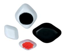
Diamond-Shaped Weighing Boats These flexible polystyrene boats have a diamond shape that flexes for easy, accurate pouring. Shallow shape and a wide, flat bottom resist tipping. Biologically inert and resistant to dilute and weak acids, aqueous solutions, alcohols, and bases. May be used with microwave moisture analyzers. Resist temperatures to 158°F (70°C). Pack of 500.
