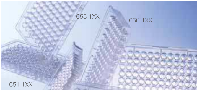
Figure 4: Well profile: 96 well F-bottom / chimney well, polystyrene Total volume: 392 µl Working volume: 25 – 340 µl Growth area: 34 mm²
