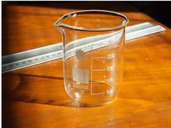
1101 Beaker, Low form with graduation and spout
