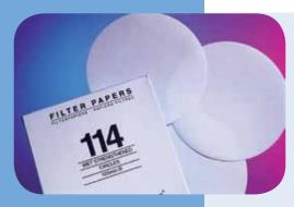
These extremely strong filter papers have a high wet strength due to the addition of a small quantity of chemically stable resin. Normal qualitative applications will not introduce any significant impurities into the filtrate. The resins do, however, contain nitrogen so these grades should not be used in Kjeldahl estimations, etc. Some wet strengthened grades are available in folded (prepleated) forms.
