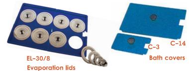
Evaporation Lids (EL) for use with WB and WBS Baths. Each Lid has openings equipped with concentric rings. The rings reduce the diameters of the openings to accommodate containers of all sizes. The El–5 Lids, for use with WB(S)–5 Baths, have four 80mm diameter openings.
