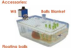
A balls blanket of Floating Polypropylene Balls is most effective for reducing evaporation and loss of heat from the Water Bath. The Balls act as effectively as a lid (flat or gabled), while enabling immersion and removal of flasks & other vessels without having to lift a lid. Usable UP to 110°C.
