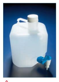
When autoclaving aspirators always ensure the caps are completely loosened or removed to prevent accidental implosion.
